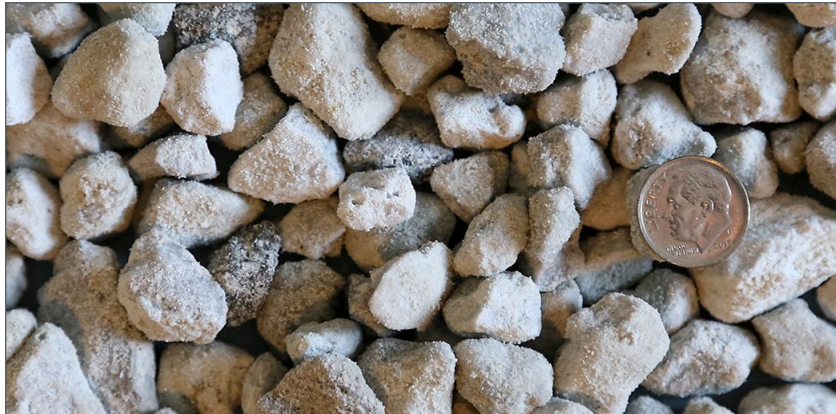
HP Grade three-quarter by three-eighths contains stones from 3/4-inches to 3/8-inches in size with some fines.
