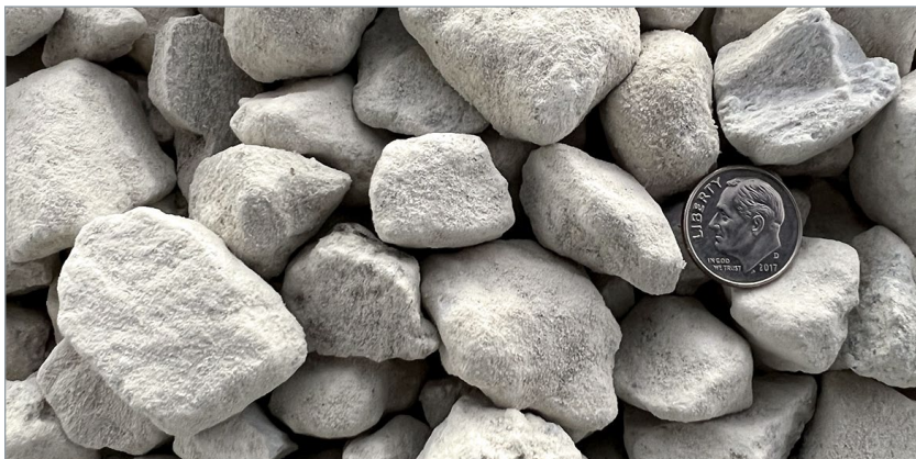
HP Grade one by three-quarters inch stones with some adhered fines.
