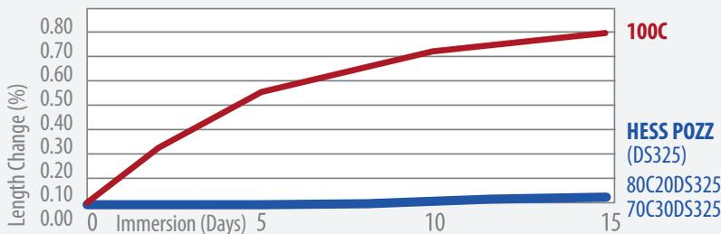
THAT GRAPH TALKS BIG. But it’s backed up with ASTM standards-research providing definitive data that Hess Standard Pozz (a natural, carefully refined pumice pozzolan) mitigates or eliminates the Alkali Silica Reaction (ASR) in curing concrete in the presence of even the most reactive aggregate. And that “pennies a yard” statement? It’s calculated by combining the savings from using less Portland cement with the cost of the HessPozz replacement.
