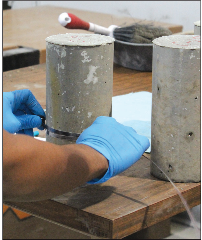
Measuring the diameter of the cylinder using a Pi tape.
