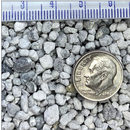
Left: HP Grade designation SBH (#10 Heavies). Right: Sand Blast Heavies used as a blast gun media.
