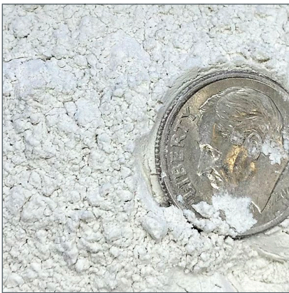
Left: HP Grade designation FFFF. Right: Grade used add a gentle abrasive to toothpastes.
