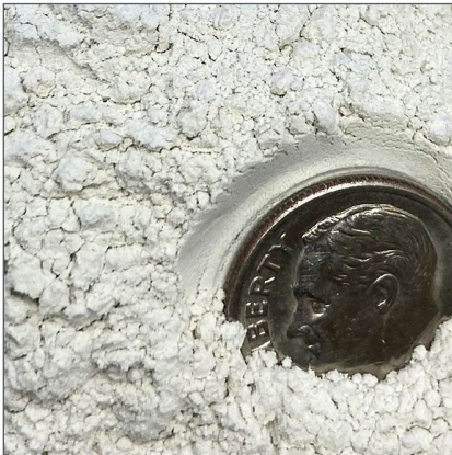
Left: HP Grade designation DS325. Right: Grade used as a supplementary cementitious material (SCM) to greatly improve concrete performance.
