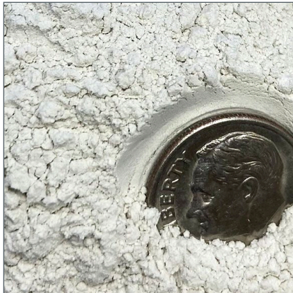
Left: HP Grade designation -325. Right: Grade used as a toothy-yet-gentle abrasive component in polishing compounds.
